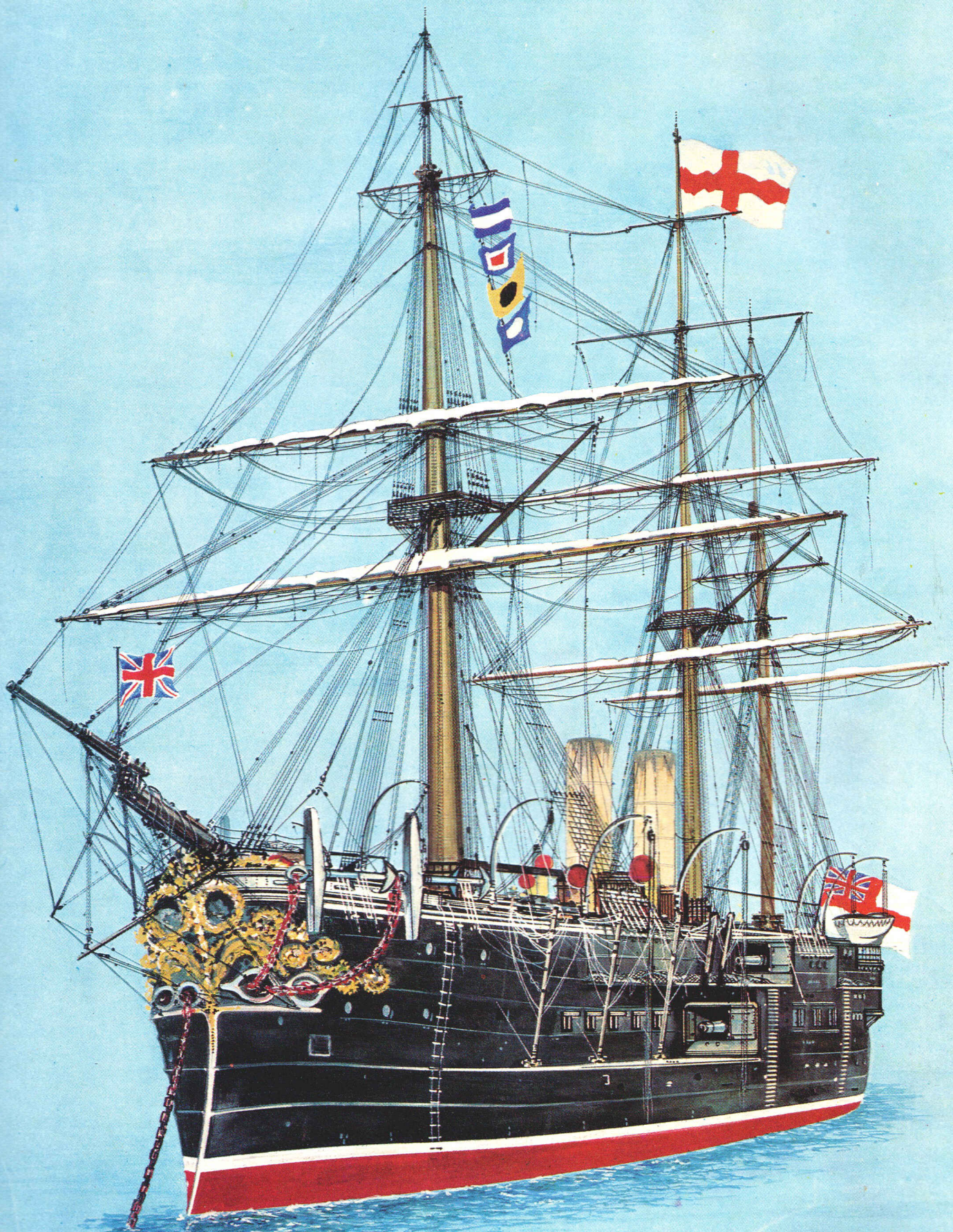
H.M.S. Alexandra , launched in 1877, was one of the last broadside ironclads to be built in Britain. Her two 11-inch and ten 10-inch guns were carried centrally below deck, and at 15 knots she was the fastest and most formidable battleship of her day.
